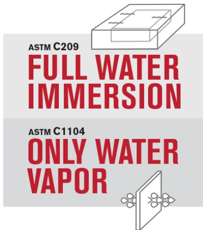
Subjecting mineral wool to the same rigorous sorption testing as polyiso proved liquid water has significant effects on mineral wool's structure and performance. When mineral wool was initially wet in accordance with ASTM C209, results showed:
